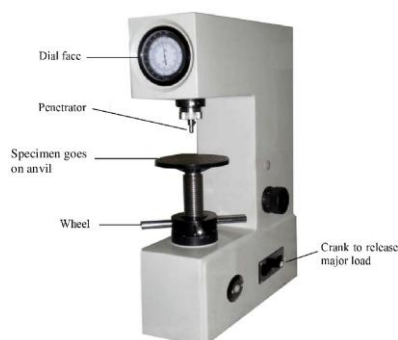
Fig. 2. Components of the Rockwell hardness tester
